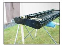
ATTACH SEAT END PLATE TO SEAT ASSEMBLY. IF HOLES IN PLATE DO NOT ALIGN WITH THE SEAT ASSEMBLY, ADJUST BY USING THE RATCHET STRAP.
