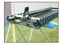
TIGHTEN STRAP UNTIL SHIPPING BRACKET BECOMES LOOSE. THEN REMOVE AND DISCARD BOLTS & SHIPPING BRACKET.
