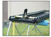
PLACE SEAT ASSEMBLY ON WORK SURFACE ALLOWING ACCESS TO ENDS. PLACE RATCHET STRAP AROUND SEAT ASSEMBLY AS SHOWN ABOVE. **1B**)
